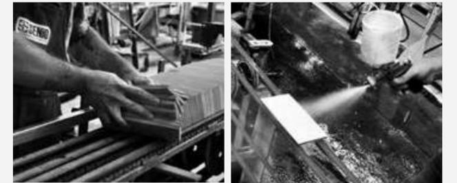
**“Double-firing”** is the process that produce Ceramics still made with earth dust, double-fired at more than 1000 °C (1832 °F) and glazed with a manual intervention, to give your wall that special natural touch of craftsmanship that other products do not have. This tile, fired twice, is the real Ceramics, understood as a blending of Earth, Glaze and Fire.
